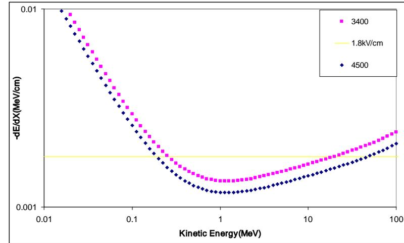
$E_{\min} = 2.14 \text{ kV/c}$  increases taking into account elastic scattering of electrons -  $E_t = 2.84 \text{ kV/cm}$
