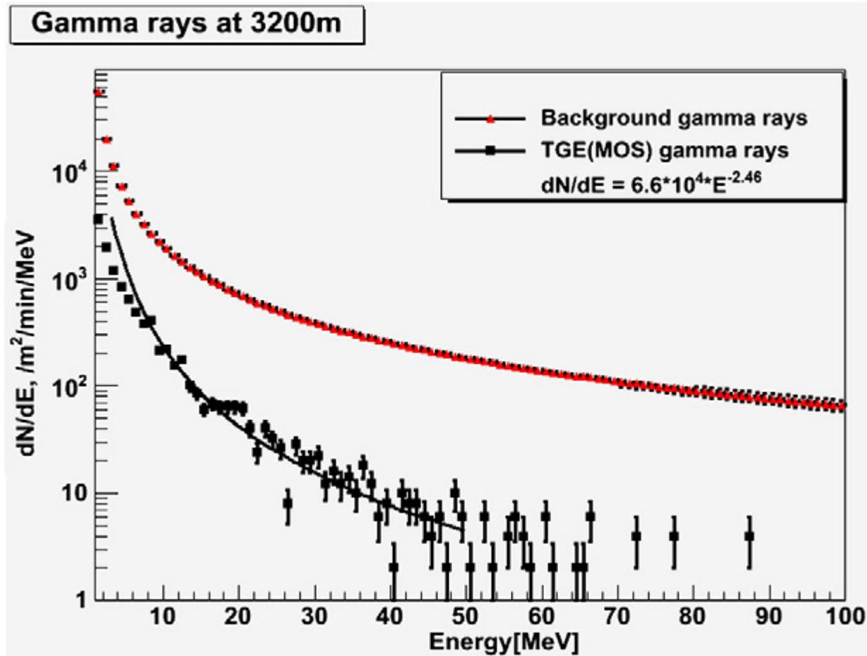
Time series of TGE of 19.06.2013.. Differential energy spectra of gamma rays measured for each separate minute. Power low indexes (\*1000) and multiplier (\*1/100) are shown.
