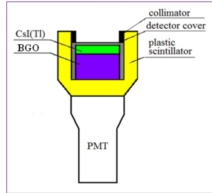
Detector consists of optically coupled thin (3mm) CsI(Tl) and considerably thick (17mm) BGO crystals with Ø20mm. Surrounding plastic scintillator is 5mm thick. FOV is formed by cylindrical collimator made of 1mm Cu.
