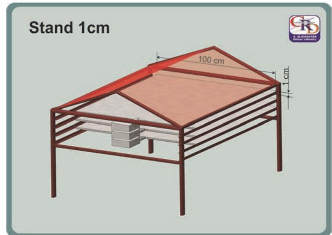
Figure 2. STAND detector consisting of three layers of 1 cm thick scintillators.
