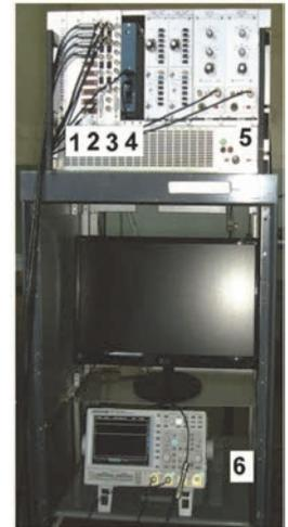
Figure 5. The LIDAR Registration and Control System.
