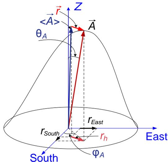
For the study of 2-dimensional variations of muon flux registered by the URAGAN, a local anisotropy vector  $\vec{A}$  is used.
