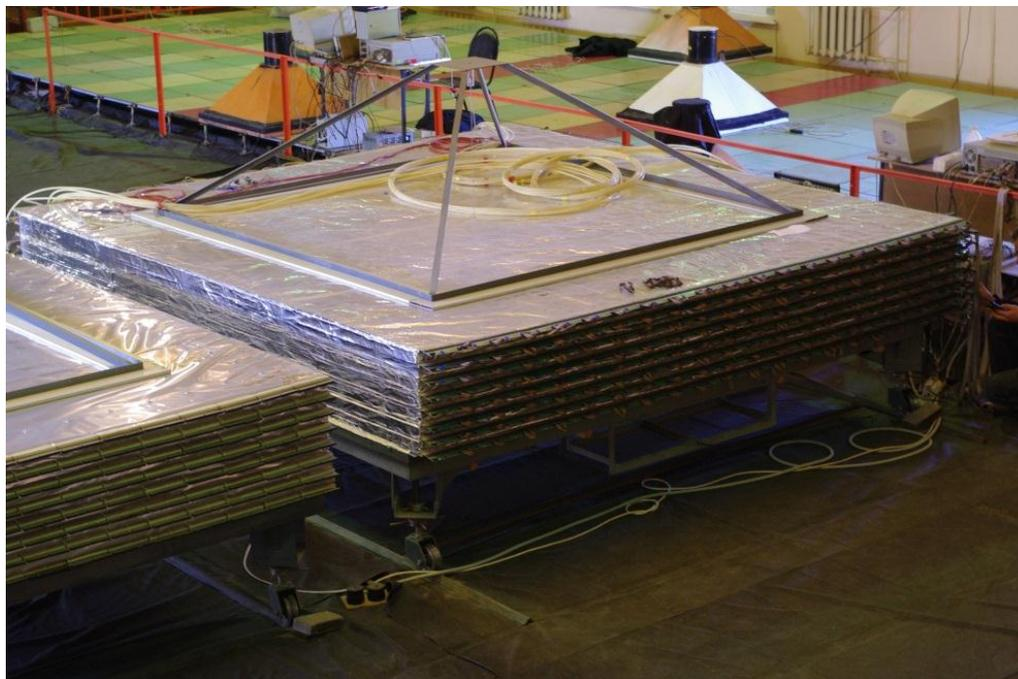
URAGAN consists of four independent supermodules (SM), total area  $\sim 46 \text{ m}^2$ . Each SM is assembled of 8 layers of gas-discharge chambers (streamer tubes) equipped with two-coordinate system of external readout strips which provides a high spatial and angular accuracy of muon track detection (correspondingly, 1 cm and  $1^\circ$ ) in a wide range of zenith ( $0^\circ$ - $80^\circ$ ) and azimuthal ( $0^\circ$ - $360^\circ$ ) angles in the real time mode.
