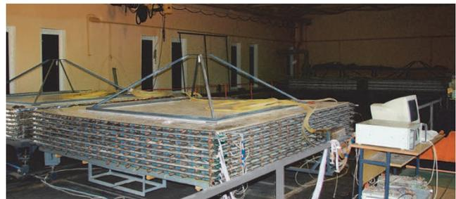
*Figure 1. The muon hodoscope URAGAN. In the foreground one of the supermodules is seen. On the left and behind, the other three SM can be seen.*
