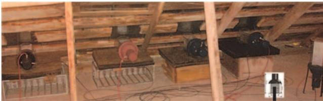
Figure 1. NaI(Tl) spectrometers installed beneath the tilt roof of the SKL experimental hall at Aragats station
