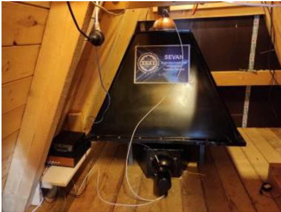
Figure 3. The final location of the SEVAN module in Kugelhime, where \approx 10 other neutron detectors are operated
