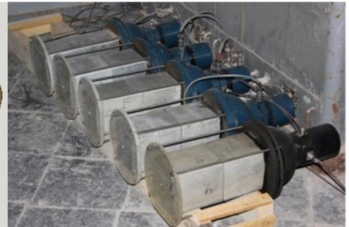
TGE electrons are registered by upper and lower layers; gamma rays and neutrons – by invoking the veto option (no signals from the upper scintillators), horizontal muons – by the condition of operation of 2 upper scintillators from 4 and no signal in the lower scintillators (to prevent registration of EAS events) and by very large energy release.
