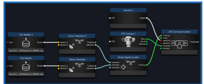
A typical setup for drone detection
