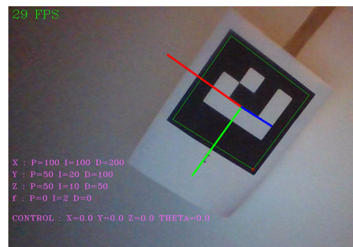
Fig. 11: Single ArUco marker with calculated vectors.
