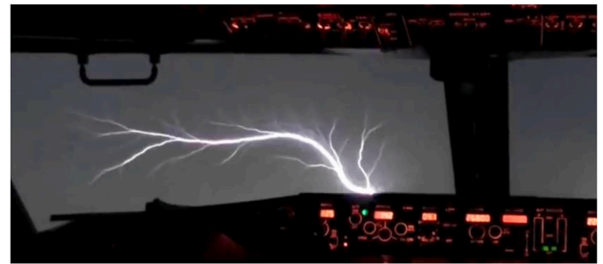
Fig. 5. Electric discharge on the surface of an aircraft window. Discharge path splitting indicates the discharge was initiated on the window frame rather than the glass. From YouTube/PilotsTubeHD, with permission.
