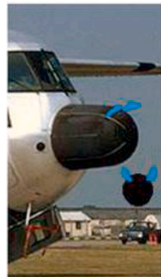
Fig. 4. (a) C-133 A cargo aircraft showing metal dividers in pilot's wind shield. (b) Shows corona "horns", marked in blue by Don Smith on black radome; Photos from US Air Force, Wright Patterson.
