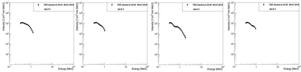
Pb<sup>214</sup> (0.3 MeV)and Bi<sup>214</sup> (0.6 MeV) decay curves measured by NaI N4 (lead filters on the top – only inclined gamma rays detected). Near surface el. field measured by EFM-100 electric mill located at SKL experimental hall
