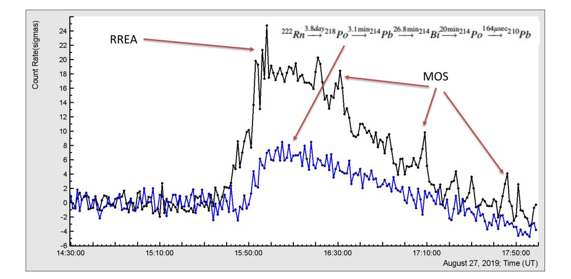
Nal 4, covered by lead on the top: no vertical gamma rays from RREA and MOS can enter it; only declined diffuse gamma rays originated from Rn progenies and lifted by the electric field to atmosphere can enter from the sides and be counted!
