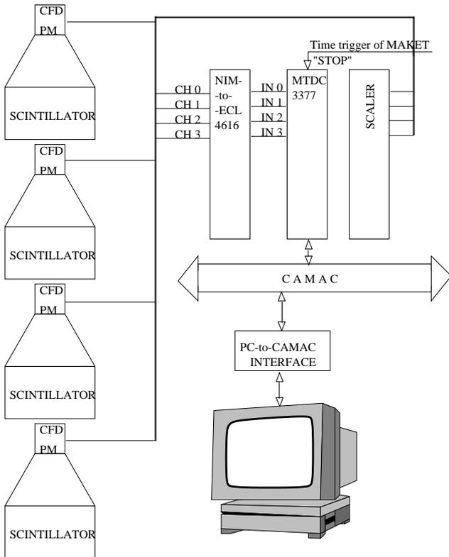
Fig. 1. A block diagram of neutron timing system.
