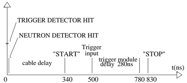
Fig. 2. A delay diagram of neutron timing system.
