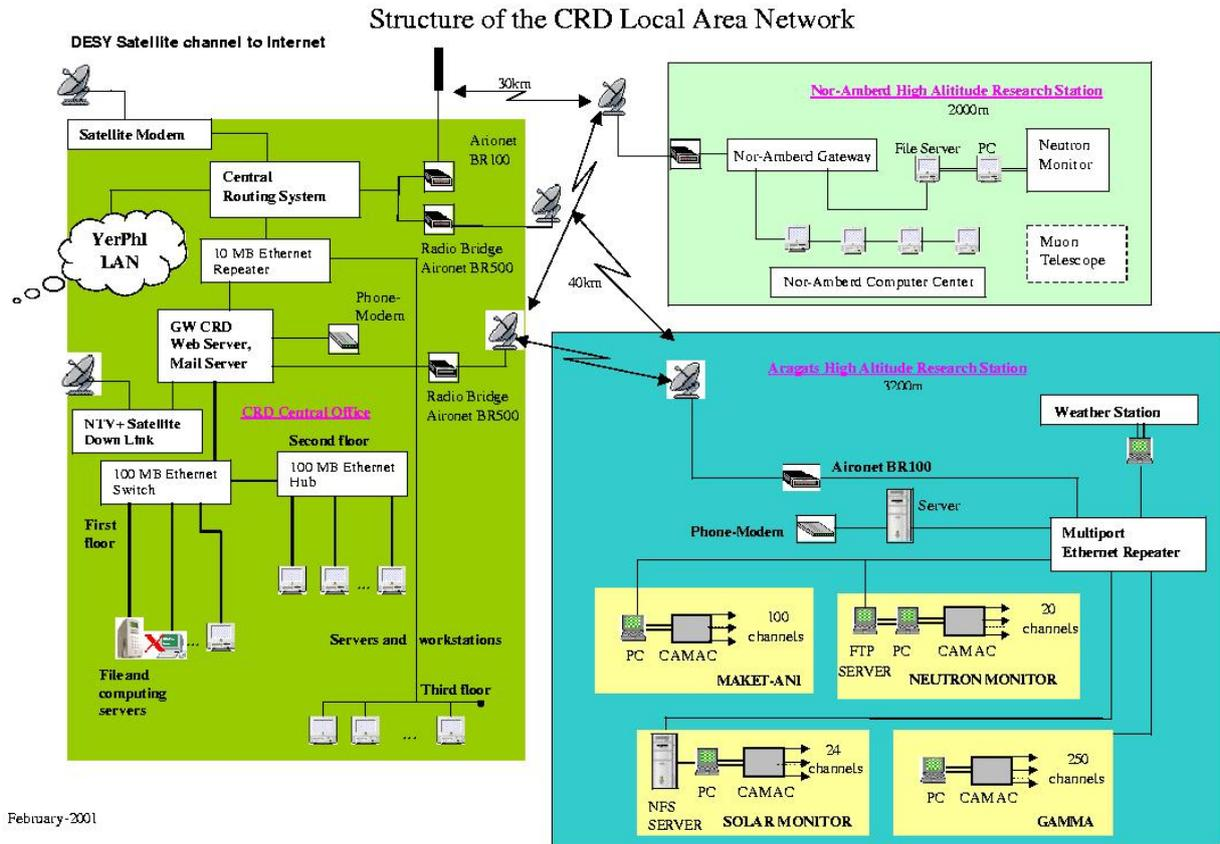
**Fig. 3.** Local Area Network and monitoring facilities of ASEC
