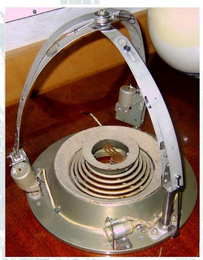
Ejection device is spring type: after command supply on separations knifes work, coupling tapes are exempted, and due to energy of a spring there is a pushing away of a satellite to speed about 2 m/s.
