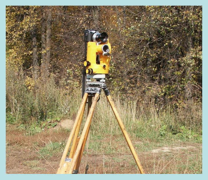
Digital camera strengthened to theodolite is used in practical work of geographers for stereo shooting when studying natural objects
