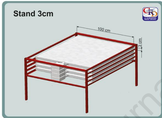
Figure 2. The Stand 3cm detector consisting of four stacked 3 cm thick scintillators with an area of 1 m 2 .
