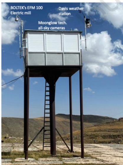
Figure 4. Electric field mill EFM 100 from BOLTEK, DAVIS weather station, and all-sky cameras installed on the roof of a small “Cuckoo’s Nest” lab.
