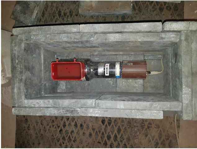
Figure 1. ORTEC firm gamma spectrometer (NaI(Tl), FWHM \sim 7.7\% at 0.6 MeV, see details in Hossain et al., 2012), surrounded by 4-cm thick lead filters. The spectrometer is positioned in the experimental hall on Mt Aragats (3,200 m MSL) which is 3-m high and located under a metallic tilt roof of 0.6-mm thickness.
