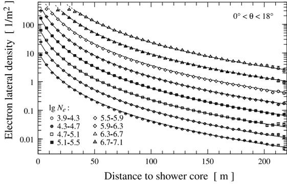
Fig. 2. Lateral distributions of electrons above a 5 MeV kinetic energy for zenith angles below 18°. The lines show NKG functions of fixed age parameter  $s = 1.65$  but varying scale radius  $r_e$  (see the text).
