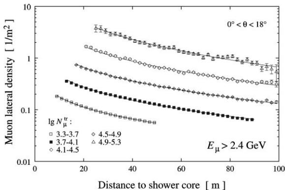
Fig. 9. Lateral distribution of muons above 2.4 GeV kinetic energy. Error bars are statistical only. Data are binned according to  $N_{\mu}^{\text{tr}}$  as measured by the array and the lines represent NKG fits to the data.
