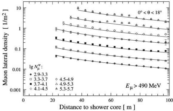
Fig. 8. Lateral distribution of muons above 490 MeV kinetic energy as measured with the trigger plane. Data are binned according to  $N_{\mu}^{\text{tr}}$  as measured by the array and the lines represent NKG fits to the data.
