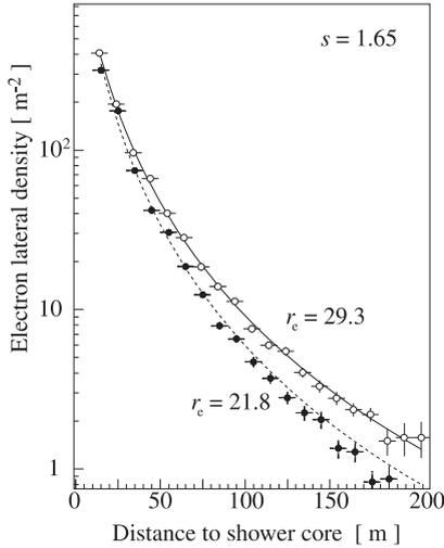
Fig. 5. Lateral distributions of two EAS events as measured by KASCADE. Both distributions are approximated by NKG functions of fixed age parameter  $s = 1.65$ . The fit parameters are  $r_e = 29.3$  m,  $N_e = 2.3 \times 10^6$  (full line), and  $r_e = 21.8$  m,  $N_e = 2.0 \times 10^6$  (---). The reconstructed zenith angles are  $\theta = 26^\circ$  and  $\theta = 30^\circ$ , respectively.
