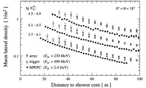
Fig. 10. Comparison of lateral distributions as measured with different KASCADE detector components for three different intervals of  $N_{\mu}^{\text{tr}}$ .
