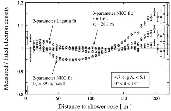
Fig. 3. Residuals in the ratio of measured over fitted average LDF with the NKG function (3-parameter fit, circles:  $N_e$ ,  $r_e$  and  $s$  free; 2-parameter fit, diamonds:  $r_e$  fixed at 89 m) and the function (4) proposed by Lagutin [10] (squares;  $N_e$  and rms radius fitted).
