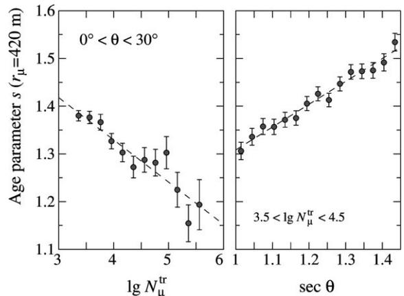
Fig. 11. The age parameter  $s$  in NKG fits with fixed  $r_{\mu} = 420 \text{ m}$  for muons of 230 MeV threshold. (a) Dependence on  $N_{\mu}^{\text{tr}}$  for zenith angles below  $30^{\circ}$  and (b) dependence on the secant of zenith angle  $\theta$ , for  $3.5 < \lg N_{\mu}^{\text{tr}} < 4.5$ . The dashed straight lines are drawn to guide the eye.
