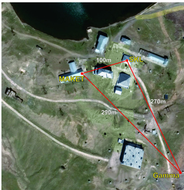
FIG. 22. STAND1 detector network. Each of the three units comprises vertically stacked three 1 cm thick and 1 m 2 area plastic scintillators and the same area stand-alone 3 cm thick plastic scintillator.
