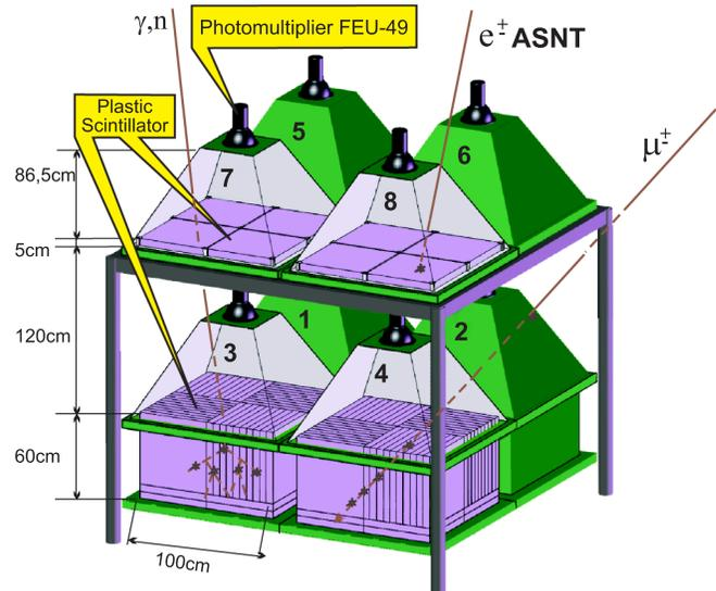
FIG. 2 (color online). Aragats Solar Neutron Telescope (ASNT).
