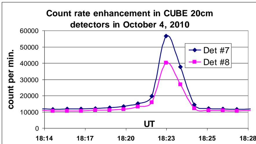
Figure 4. Count rate enhancement of Cube inner scintillators; October 4, 2010
