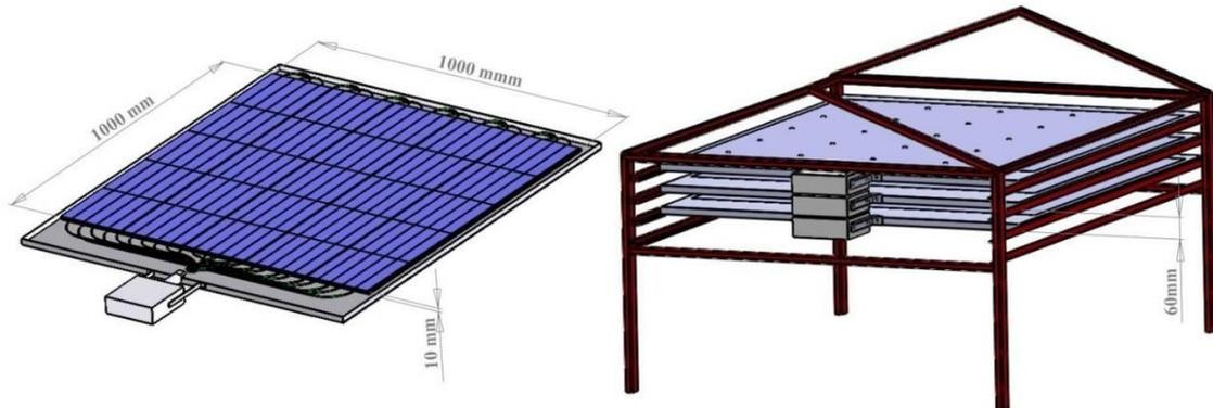
Figure 1. Stand assembly and design of 1 cm thick molded plastic scintillator with optical spectrum-shifter fibers; details of detector construction see in [2].
