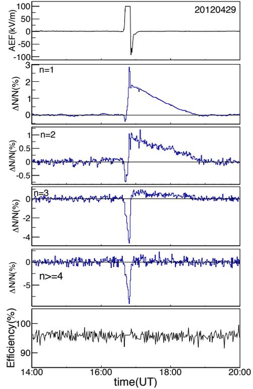
**Figure 2:** The thunderstorm event (20120429) between 14:00 and 20:00 UT on April 29, 2012. From top to bottom, the AEF value, the percent variations of counting rate for  $n=1$ ,  $n=2$ ,  $n=3$ ,  $n \geq 4$  and the efficiency of the detectors are shown. The counting rate data from 14:00 to 16:00 and from 19:00 to 20:00 are considered as background, averaged every minute.  $\Delta N$  represents the difference between the data and the mean value  $N$ .
