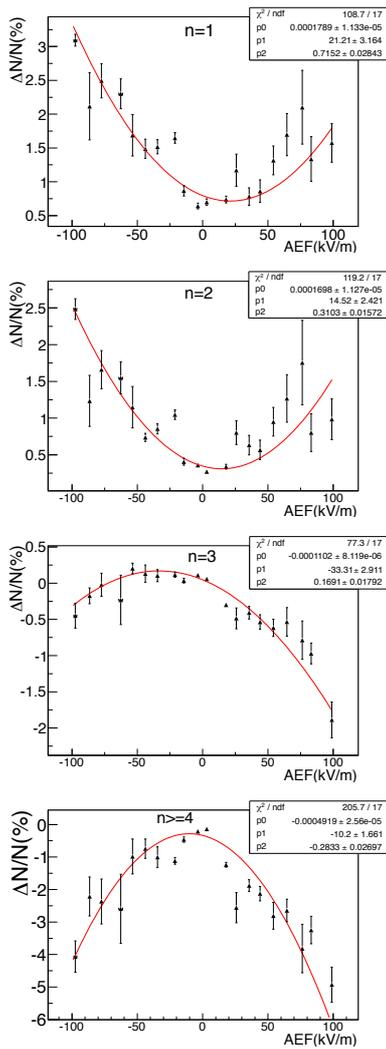
**Figure 5:** The amplitude of the counting rate relative variation versus the electric field strength. Observations of 24 thunderstorms are included in the analysis. From top to bottom, they correspond respectively to  $n=1$ ,  $n=2$ ,  $n=3$  and  $n \geq 4$ .
