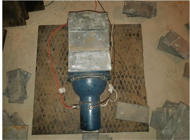
FIG. 7. NaI spectrometer (N4) covered with lead bricks (4 cm) to prevent registration of the near-vertical RREA.
