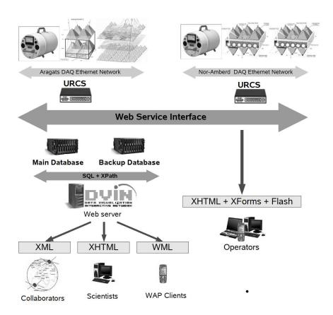
**Figure 1.** The figure represents a layout of the new ASEC data acquisition system. Several detector arrays are operating at Nor-Amberd and Aragats research stations. The detectors are controlled by URCS which are installed on each station. The data dissemination and detector control is facilitated by web services. The DVIN is used to distribute the data to end users.
