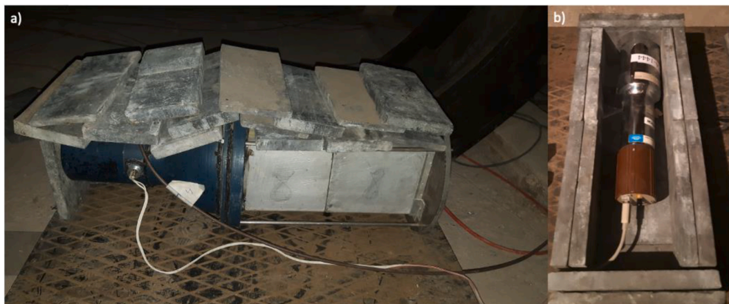
Fig. 2. Large NaI spectrometer with lead filters above a); ORTEC spectrometers with lead filters from the sides and the bottom b).
