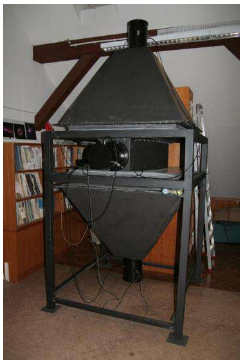
Figure 3. SEVAN Particle Detector for Solar Physics and Space Weather research placed on Zagreb Astronomical Observatory.
