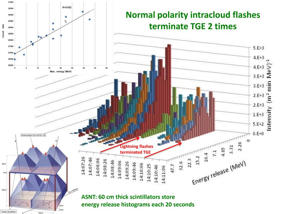
Correlation of gamma ray flux intensity and maximal energy (in strong electric fields avalanches are both intense and energetic).
